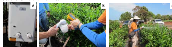
Figure 2: A) The portable gas powered tankless water heater, B) infrared thermometer is used to measure the hot water temperature in a measuring cup, and C) tea plants were sprayed with a portable water heater and spray nozzle.
